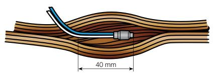
The transition to the heavier lead wire should take place within the end coil lacing, since mechanical stress during manufacture and final assembly ("robust" handling) or vibration during compressor running could lead to an open circuit.
